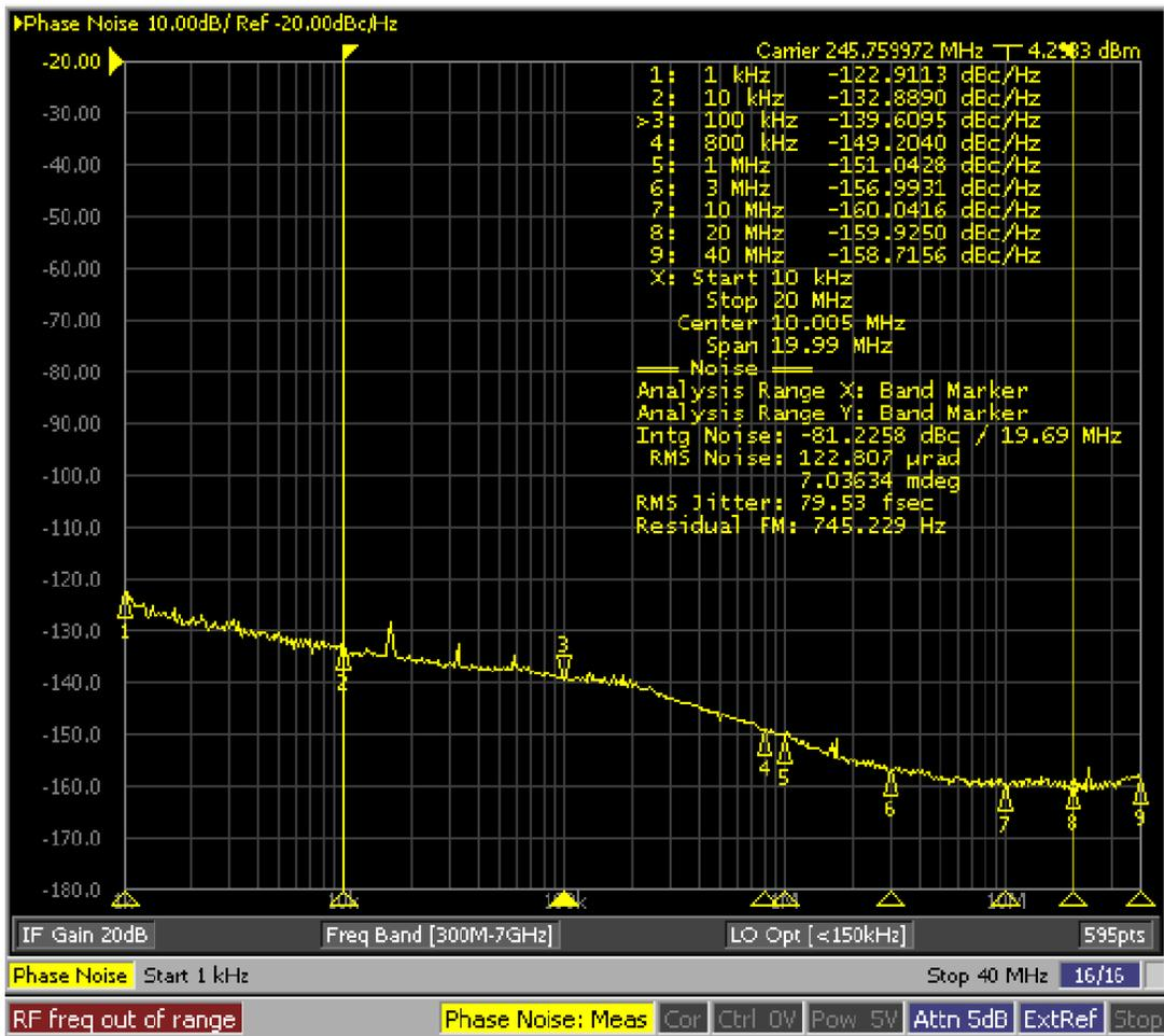
VCO\_MUX = 0 (VCO0)    PLL2 Loop Filter Bandwidth = 344 kHz
