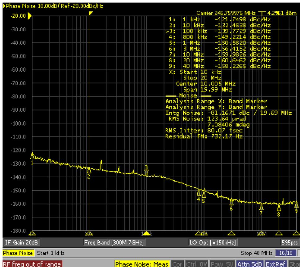
VCO\_MUX = 1 (VCO1) PLL2 Loop Filter Bandwidth = 233 kHz
